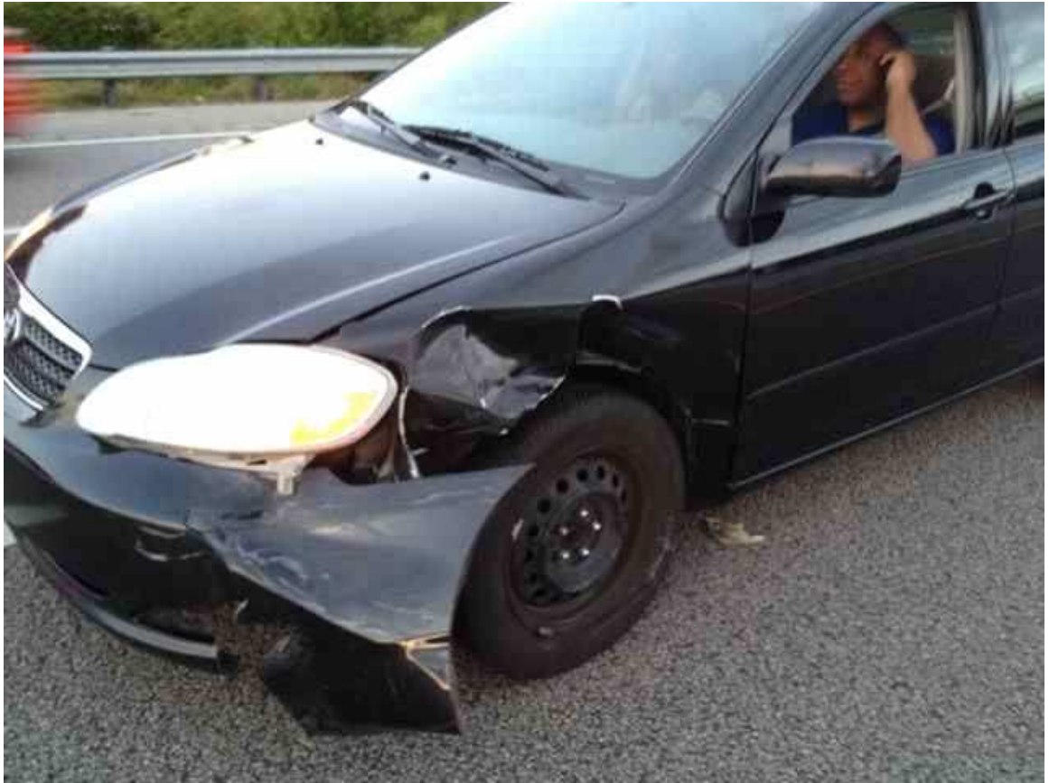
Damage to car 3 confined to left front quarter panel and bumper. No other damage occurred.
