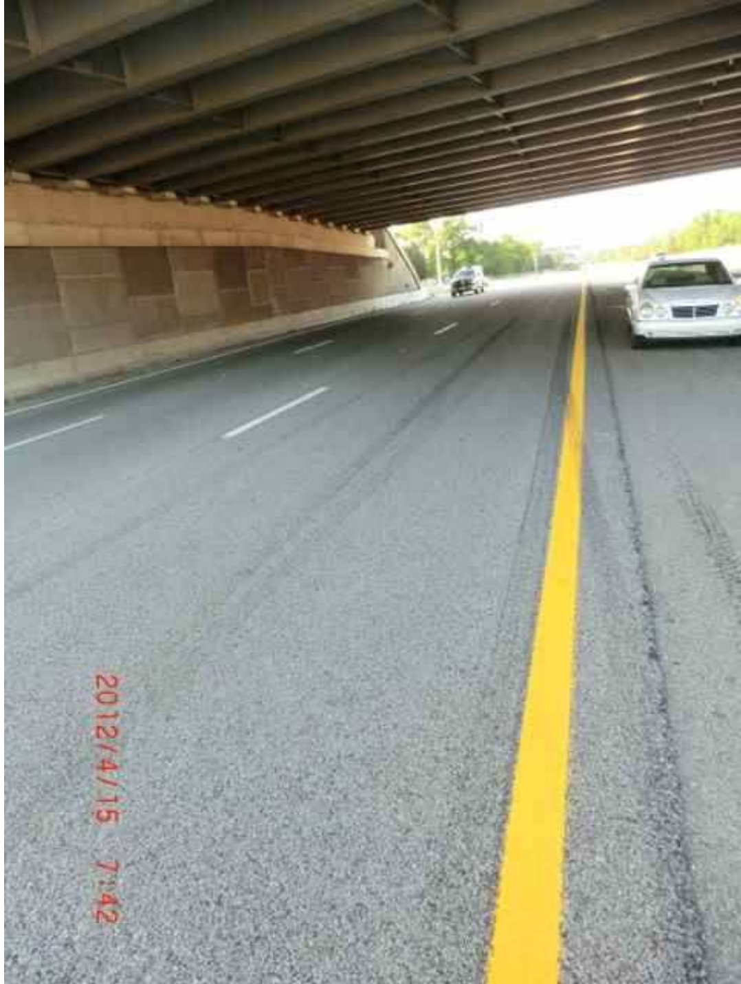
Photo: Start of accident skid marks. Note two sets of skids and position under the bridge ~190 ft from on ramp (where the truck is entering the highway).
